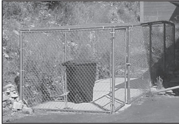
If you can't store your garbage inside a sturdy, locked building, a heavy-duty chain-link fenced enclosure with a chain-link "roof," concrete pad bottom, and locking (not latching) gate can help keep out your average bears — but smells will still attract them, as well as other wildlife, so you will need to be extra vigilant and make sure there are no other food sources around.
